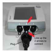
When connected to the device, plug the AC cord into the other end of the charger and then into a 110-120V outlet. At first you will see a red light on the charger. After about 3 hours it will turn a steady green color when charging is complete.
