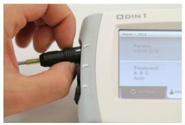
When the treatment is complete, the device will automatically shut itself off. Once that has occurred, firmly grasp the patient cables on the sleeve portion of the plug and pull straight back to remove from the device. You should feel the sleeve slide back and the locking mechanism disengage. **Do NOT twist the plug or pull from the back shell or wire to remove.**
